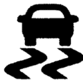
Figure 3: ESC Malfunction Telltale Symbol in FMVSS No. 101
