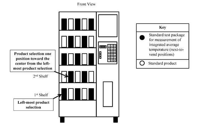
Figure B.1. Location of Standard Test Packages for Refrigerated Bottled or Canned Beverage Vending Machines with Products Arranged Horizontally and Five Next-to-Vend Product Locations on Each Shelf.
