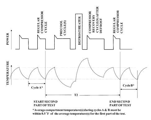
4.2.1.2 Non-cycling Compressor System. For a system with a non-cycling compressor, the second part of the test starts at a time before defrost during stable operation when compartment temperatures are within 0.5  $^\circ\mathrm{F}$
