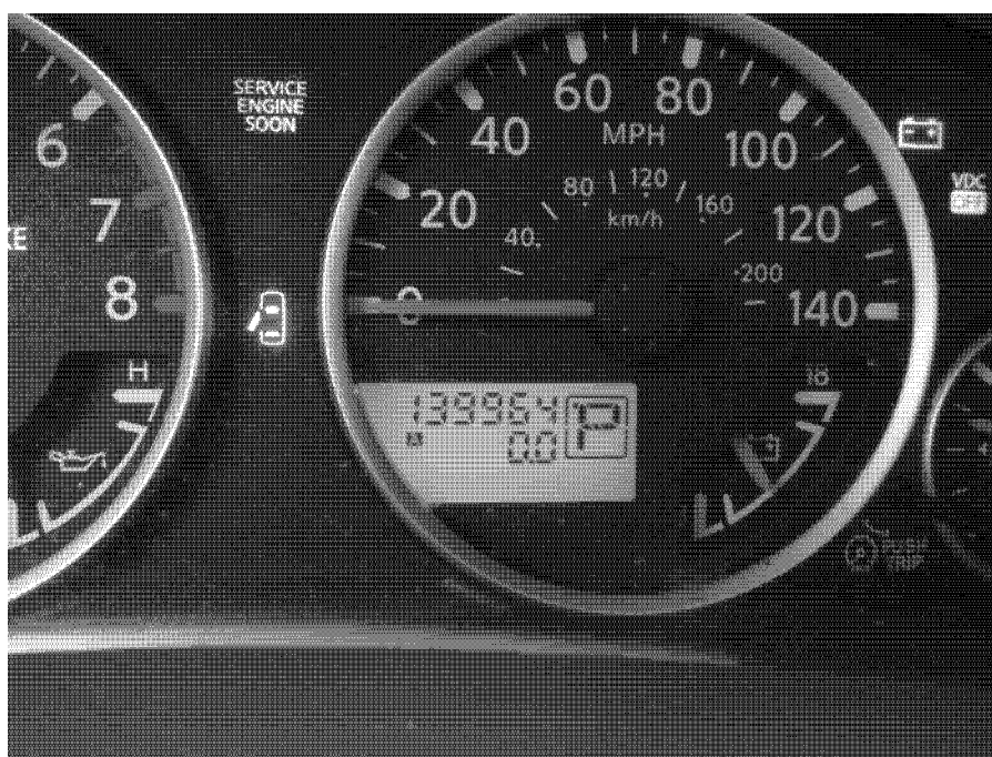
Photo 4 – Subject vehicle MIL - "Service Engine Soon"
