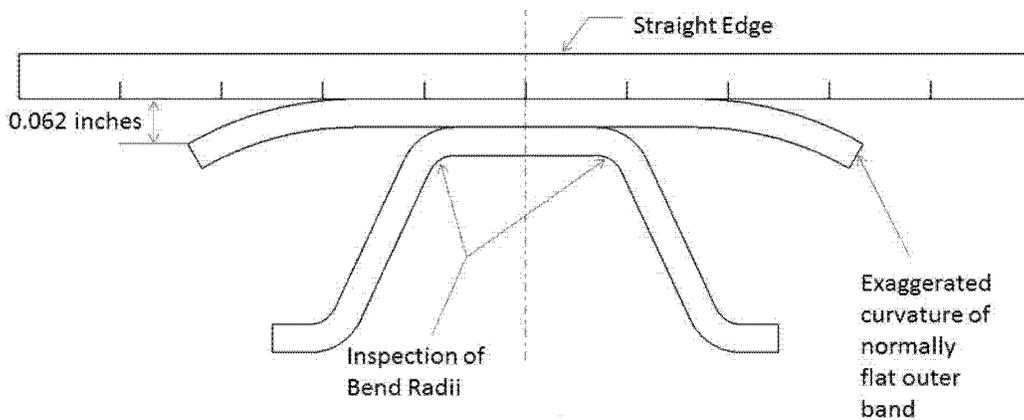
Figure 1 to paragraphs (h)(1)(iii) and (v) of this AD: Cross section of v-band coupling
