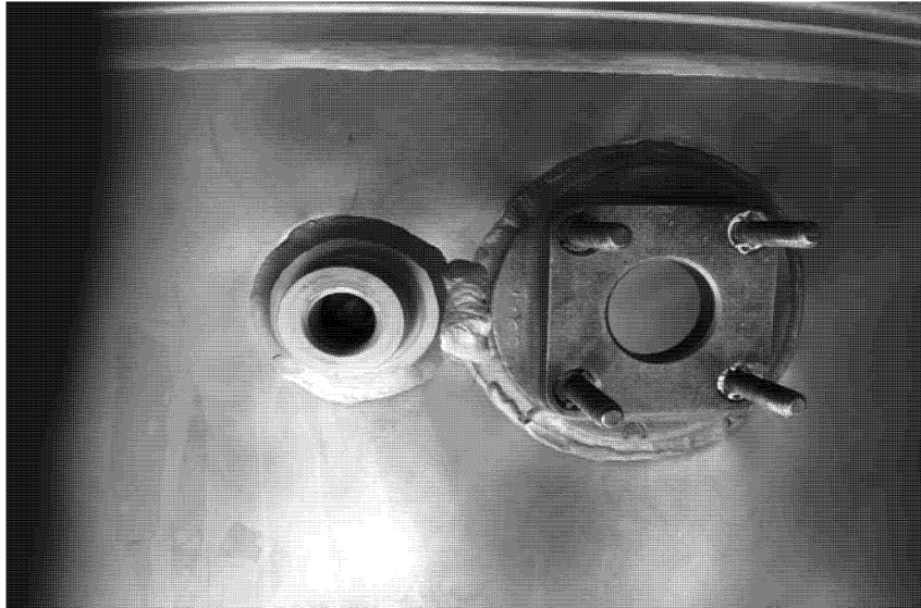
Figure 2 to Paragraph (h) of this AD. Combustion Chamber Case Assembly with One-Piece Bleed Pad with P3 Boss
