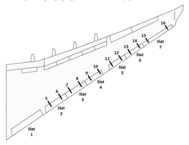
**Figure 2 to paragraph (g) of this AD** – Affected Slats, Slat Track Positions, and Part Numbers (P/Ns)
