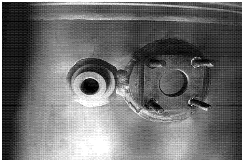
Figure 1 to Paragraph (h) of this AD. Combustion Chamber Case Assembly Without the One-Piece Bleed Pad with P3 Boss
