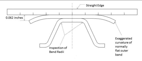
Figure 1 to paragraphs (k)(1)(iii) and (v) of this AD: Cross section of v-band
