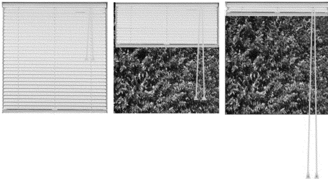
Figure 12. Window covering showing the length of the free hanging operating cord in three positions: fully lowered, middle height, fully raised.
